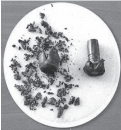
Figure 9(b): A photograph showing the difference between a lead (left) and a non-lead bullet (right) after impact
